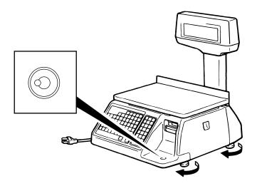
② When the air bubble moves toward rear, turn the front adjustable legs clockwise.
